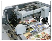
mechanism feeds individual sheets into the SmartStacker for finishing.
