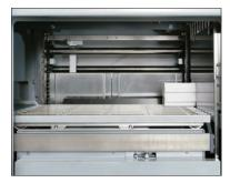
Maximum stack height is 254 mm / 10". Stacked sheets are delivered to the output conveyor for easier handling or downstream finishing.
