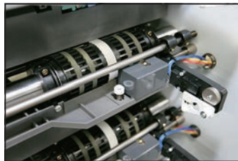
Suction feed section on a bin Stable feeding capability for a wide range of sheets.
