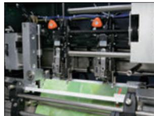
Booklets up to 10 mm thick (50 sheets of normal 80 gsm paper) can be stitched. The folded sets are jogged from the head and foot, then centered on the saddle by the centering mechanism before the heavy-duty stitching heads fire to produce accurately stitched booklets.
