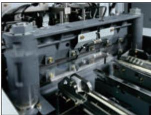
The servo-motor controlled feed mechanism provides for accurate booklet registration and fore-edge trimming. The guide is automatically adjusted according to the sheet size input on the touchscreen on the SPF-30S.
