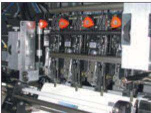
Standard stitcher head (#24 to #26 - thickness: 0.6 mm to 0.5 mm) and optional stitcher head (#26 to #28 - thickness: 0.5 mm to 0.4 mm) are available. Additional stitcher heads are available for up to 4 stitches per booklet with mounting block B-30S.
