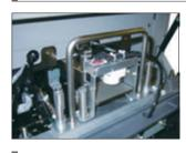
The HTS-TD is installed at foreedge trimming section and checks the thickness of each booklet. In case of missing section or double sections, system stops for maximum quality control.
