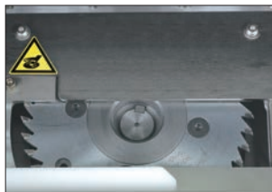
Leveling Cutter: Mills the book spine. Notching Cutter: Cuts grooves on the book spine to insure strong book binding.
